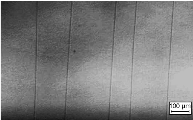
Fig. 3. Through-thickness surface cracks across tensile surface of two-step ion-exchanged glass four-point-bend specimen at 210 MPa applied stress (fine surface finish).
